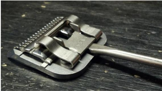
To fix the blade to work on your Furzone clipper is very simple and easy. All you need is a flat head screwdriver. Just stick the screwdriver into the back of the socket as shown, then slightly TWIST the screwdriver, DON'T TRY TO PRY IT. You just want to twist it enough so you think it moved up a little. Then try it on the clipper, if it doesn't fit, twist it a little more.
